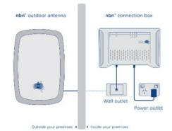
This is the most common technology for rural areas or whenever is not possible to use any other technology. An external antenna is connected with fibre optic to the NTD, which should be inside the premises, which looks like the image above.
